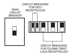
Figure 69. Main, Aux. and GFCI Circuit Breakers (OFF)
